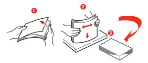
**3.** Load paper long edge feed (LEF) (for letterhead paper load face down with top edge towards the right of the unit) (1) up to mark (a).
